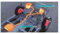
SELF CHARGING BATTERY The Swift's ISG uses decelaration and braking energy to efficiently recharge the Swift's lithium ion battery, so there's no need to worry about plugging in.
