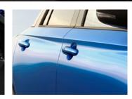
**KEYLESS ENTRY AND START** Enjoy seamless access to your Swift while the keys stay safely in your pocket or bag. Unlock the door while pressing the button on the door handle. and start the car with just one push.
